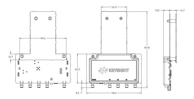
The N2135A 3-in-1 programmable NFC antenna provides 15 mm spacing between poller/listener coils.
