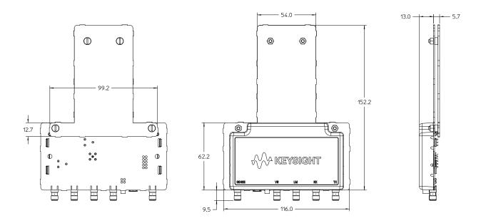
The N2116A 3-in-1 programmable NFC antenna provides 5 mm spacing between poller/listener coils.
