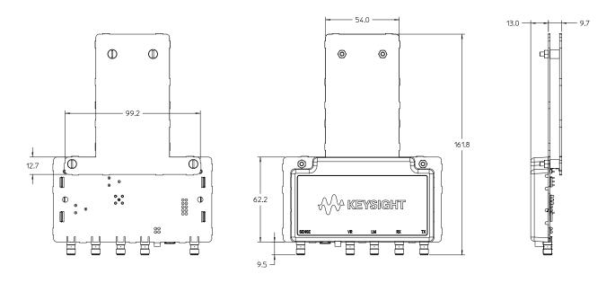
The N2134A 3-in-1 programmable NFC antenna provides 10 mm spacing between poller/listener coils.
