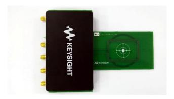
The TCI-II programmable NFC multi-coil antenna includes a Poller 3 and Listener 3 equivalent test antenna that can be quickly switched between various test modes for fast test throughput. The following shows a block diagram of Keysight's TCI-II programmable NFC antenna.
