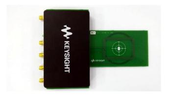
The Keysight 3-in-1 programmable NFC multi-coil antenna includes a Poller 3 and Listener 3 equivalent test antenna that can be quickly switched between various test modes for fast test throughput. The following shows a block diagram of the Keysight N2116A, N2134A, and N2135A 3-in-1 programmable NFC antennas.
