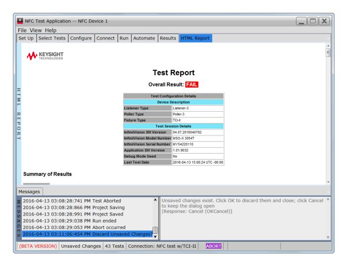
The NFC Test Application provides complete report generation with statistical and margin analysis capabilities. NFC test results shows Poller/Listener parameters that fail to meet specifications highlighted in red, as well as marginal test results highlighted in yellow.
